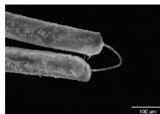
Fig. 2 SEM micrograph, showing a bottom view of the Wollaston wires and the 5 \mu\text{m} diameter platinum-rhodium filament used in \mu\text{TA} as thermal element
